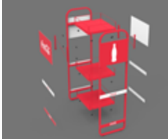
Disassemble option 8% cost reduction 4x reduced volume
